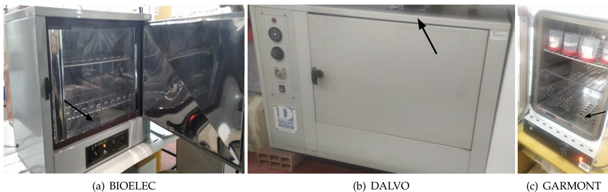
Figure 1. Examples of microbiological incubators and their temperature sensors positions indicated.
