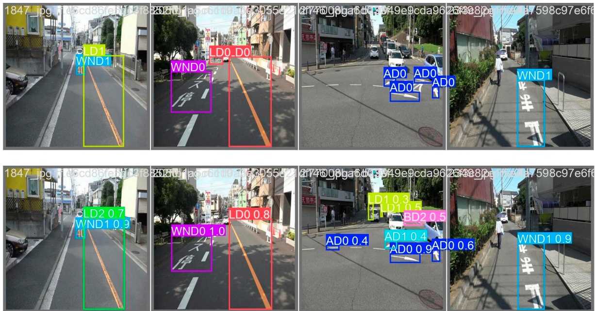
Figure 12. Visualization of road marking damage detection results of YOLOv11x on four test images (first row: ground truth; second row: results of prediction).
