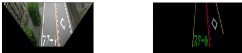
Figure 4. Examples of the obtained BEV images ( left : original image; right : segmentation result).
