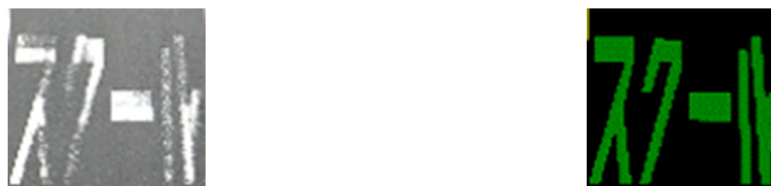
Figure 5. Examples of the cropped road marking images ( left : original image; right : segmentation result).
