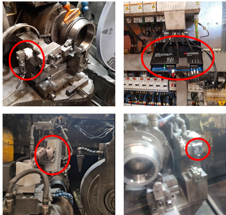
Figure 3. Sensors in the figure framed with a red circle: ( upper left ) accelerometer (PCB Piezotronics with a frequency range of 0.5 to 8000 Hz); ( upper right ) Equipment for grinding power acquisition; ( lower left ) thermal camera (FLIR Lepton 3.5); ( lower right ) AE sensor (Steminc 20 × 1 mm 2 Mhz R).
