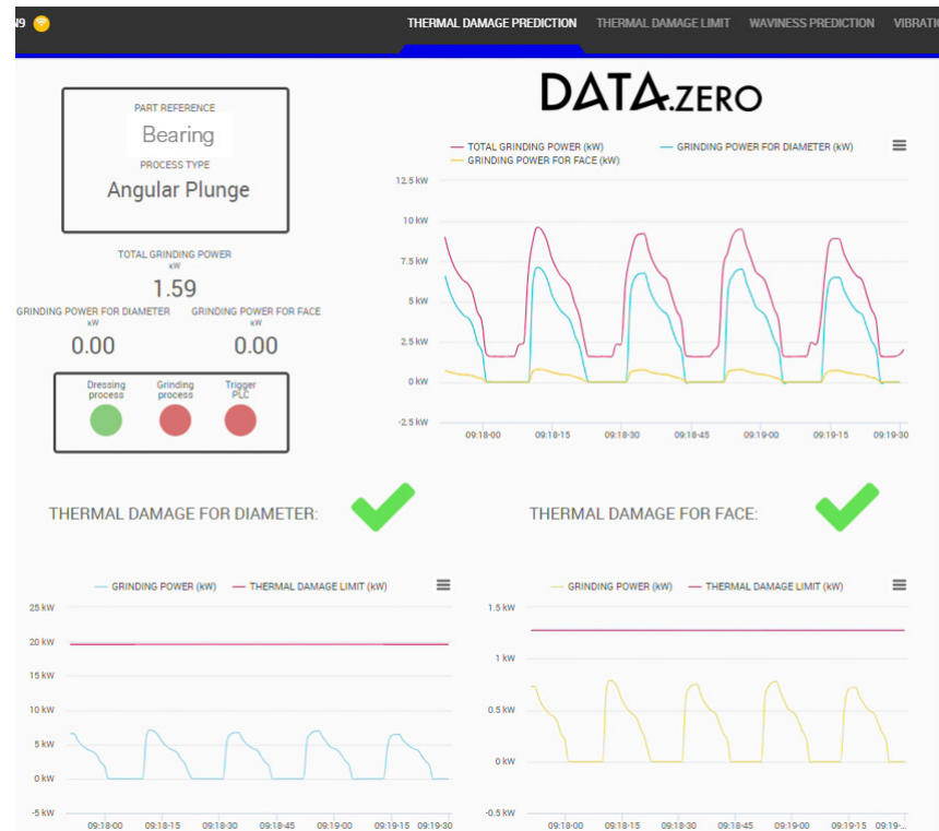
Figure 18. Example of the interface for the grinding quality control.
