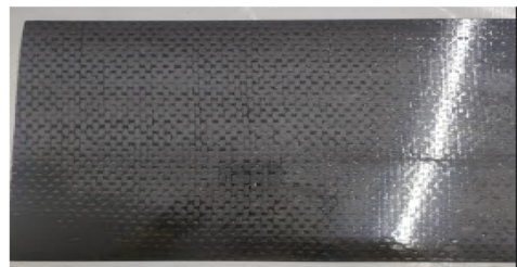
Fig. 1. Hybrid composites based on polymers reinforced with carbon fiber and epoxy resin.
