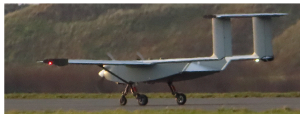
FIGURE 1 ULTRA self-flying cargo UAV (Windracers, 2023), one of the biggest UAVs in the UK, capable of carrying 100 kg of payload.
