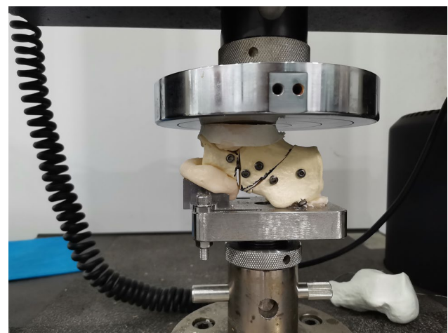
Fig. 12 The compression fixture was connected to the testing machine
