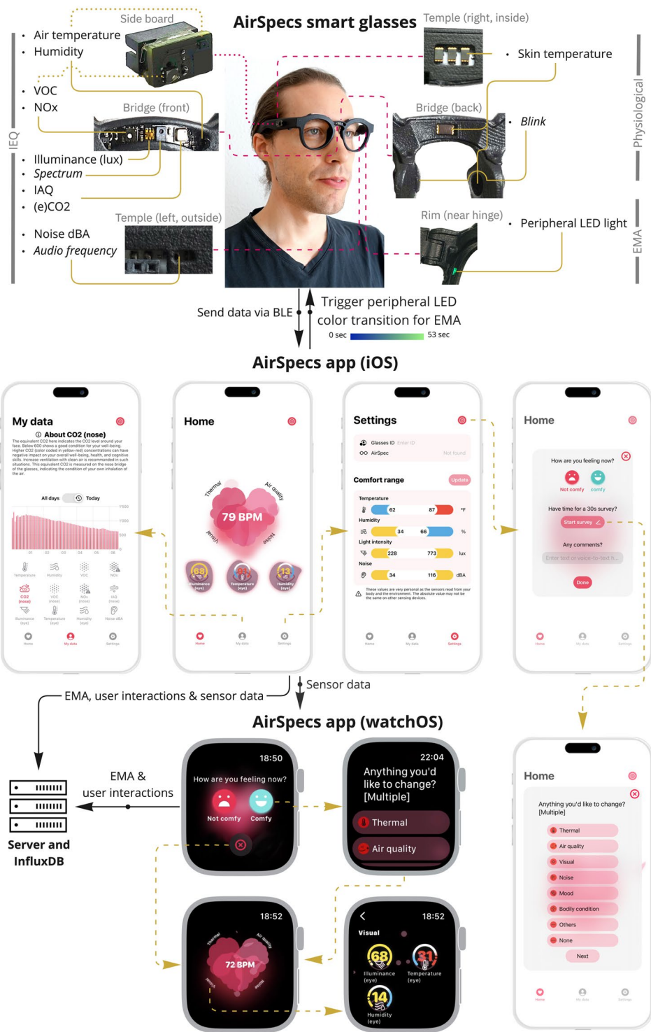
Fig. 2 System overview of AirSpecs device and apps. The sensor readings of the device in the top figure (except those in italic ) are accessible by the user. Most readings are presented in raw form, except that skin temperature data was used to estimate cognitive load. Screenshots of the AirSpecs apps design in iOS and the corresponding watchOS are shown, including home, historical records, settings, and the survey. The watchOS app aims to provide spontaneous information, so we eliminated the historical records and settings screens in its design. Two sets of sensors that measure air temperature, humidity, VOC, and NOx are located in the left temple (on a sideboard) and bridge, considering that measurements near the breathing area and the surrounding environment can differ.
