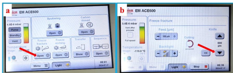
Figure 6. Setting the height of the cold knife. a. Selecting the freeze-fracture module from the main menu. b. Setting the height of the cold knife.
