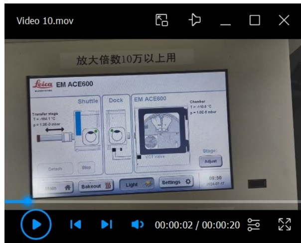
Video 10. Retrieving the cryo-stub from ACE600 back to the shuttle
