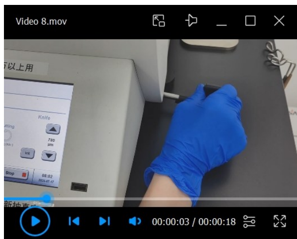
Video 8. Freeze-fracture of the samples with cold knife
