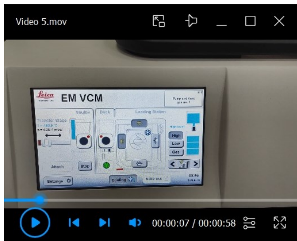
Video 5. Retrieving the cryo-stub from the VCM to the shuttle
