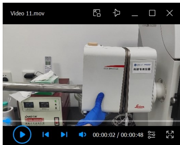
Video 11. Transferring the cryo-stub from the ACE600 to the cryo-stage of SEM
