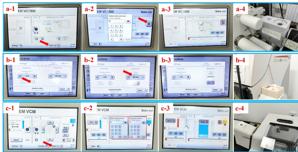
Figure 11. Baking out all the equipment. a. VCT500. b. ACE600. c. VCM and the shuttle.
