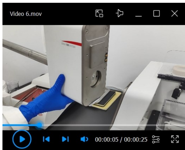
Video 6. Removal of the shuttle from the VCM and its attachment to the ACE600
