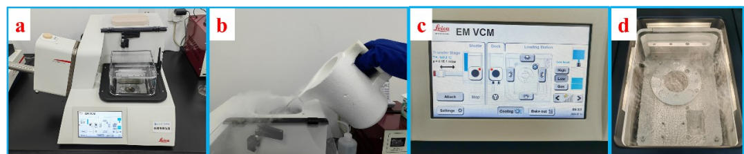
Figure 4. Overview of the VCM and preparations for cryo-fixation. a. Picture of VCM with the shuttle attached. b. Filling liquid nitrogen into the reservoir of VCM. c. Control panel of VCM. d. Liquid nitrogen bath ready for cryo-fixation.
