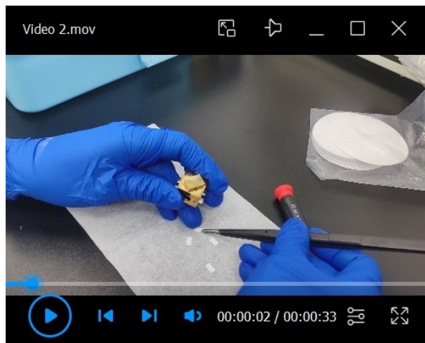
Video 2. Fixation of the filter paper strips onto the sample holder
