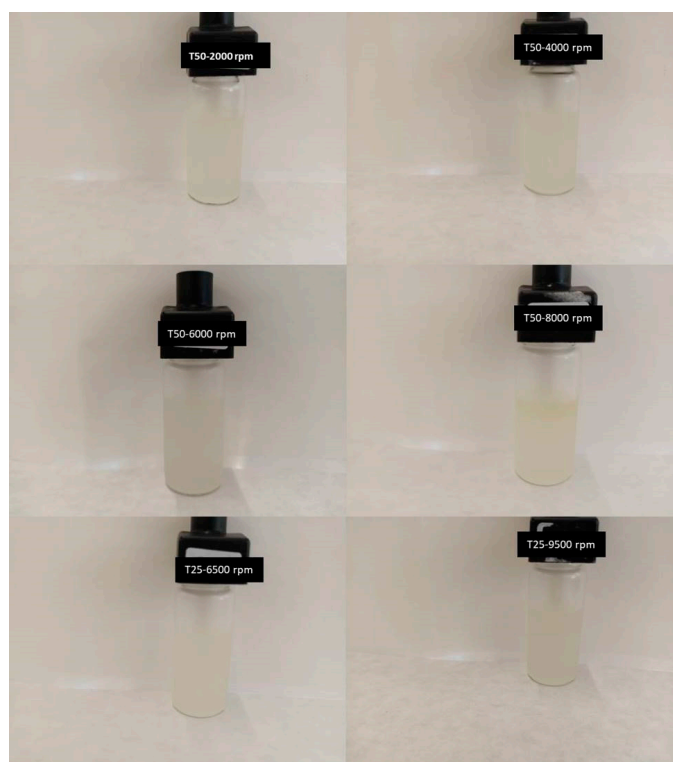
Figure 9. Visual inspection results of aqueous dispersions of flaxseed fiber three months after preparation.
