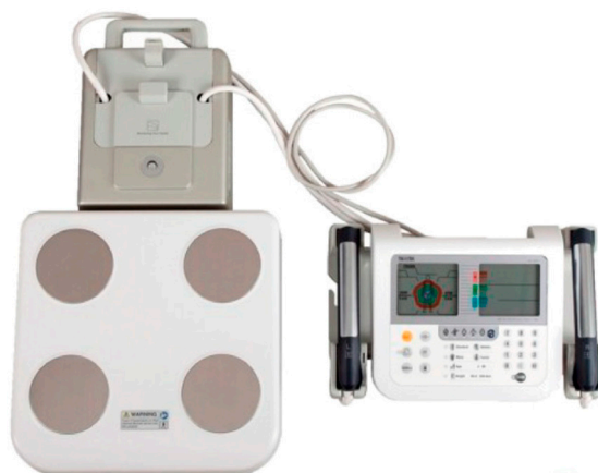
Figure 2. Picture of the bioimpedance meter “MC-780A TANITA” used for the study.
