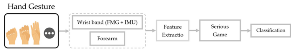
Figure 10. Wearable multimodal rehabilitation utilizing serious games involves extracting kinematic data. Relevant features are identified and input into classification algorithms to predict movements that serve as inputs for the game.
