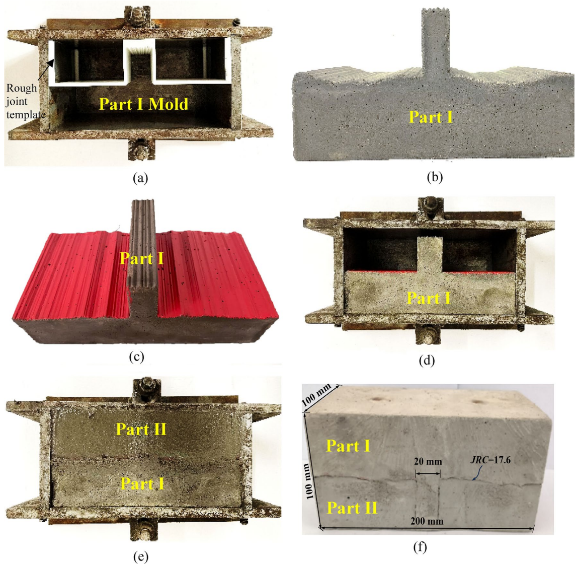
Fig. 4. The fabricating procedure used for specimens.
