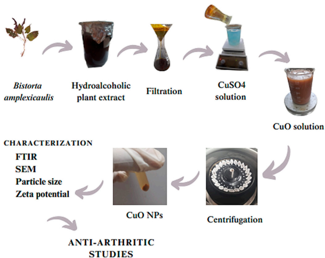
FIGURE 2 Step-by-step flowchart of the synthesis of CuO nanoparticles.
