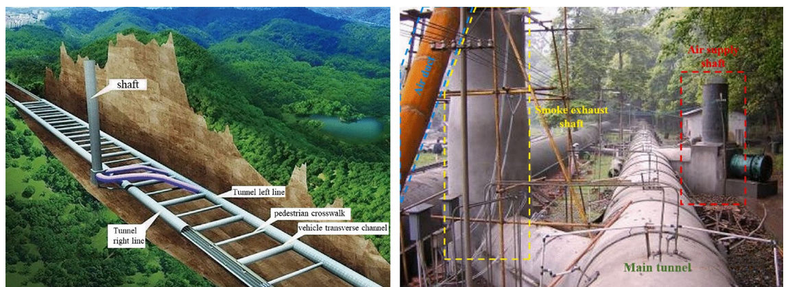
Fig. 1. Schematic diagram of a mountain tunnel with a lateral open shaft 3,4 .
