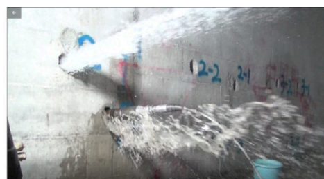
(a) Water sprayed from adjacent holes during granite testing.
