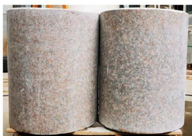
(b) Granite sample with compressive strength of 80 MPa
