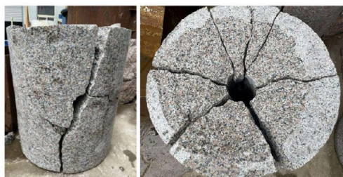
(c) The results of the gray 3 sample after 6 impacts with 70 kJ energy.
