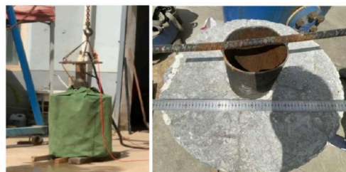
(b) High strength physical model samples with sleeves
