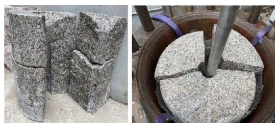
(a) The result of two impacts of 100 kJ energy on the gray 1 sample.
