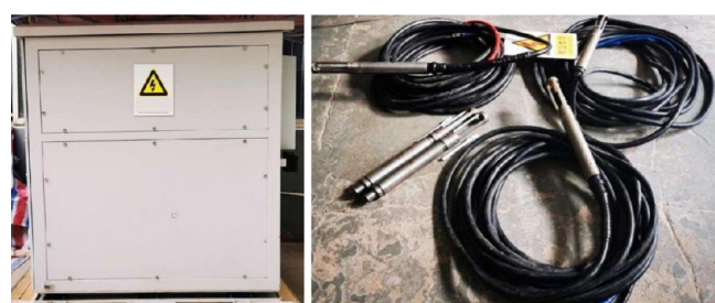
(a) 3 \times 40 kJ pulse power driving source
