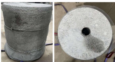
(c) Granite sample with compressive strength of 130 MPa
