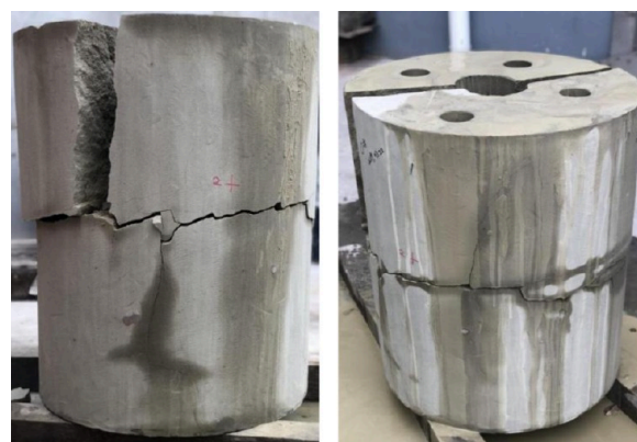
Figure 16. Sandstone samples after shock wave fracturing.
