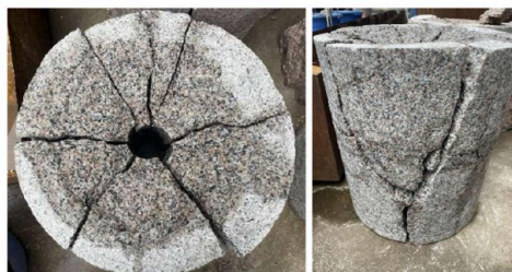
(b) The result of 6 impacts of 50 kJ energy on the gray 2 sample.
