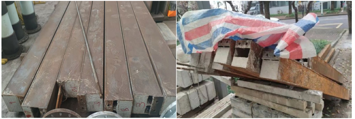
Fig. 1. Concrete-filled rectangular steel Tube beam specimens.
