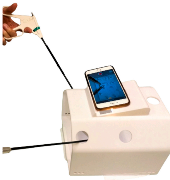
Fig. 2. Full assembled SCLT with instruments and Smartphone.
