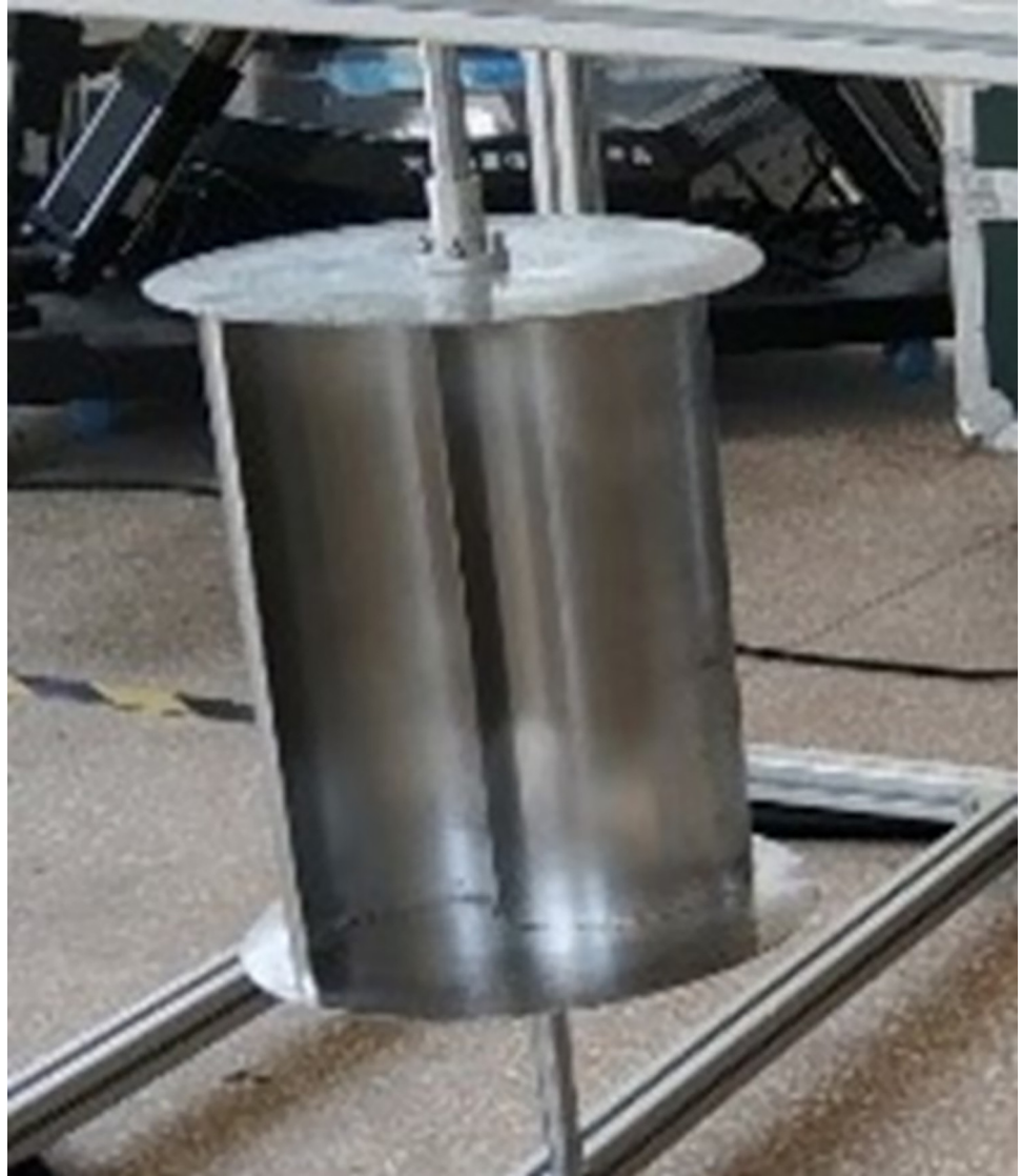
Fig 2. Physical model of the blade group.
