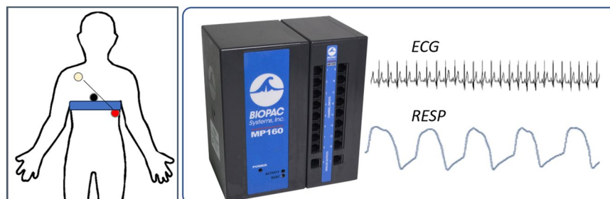
Fig. 1 Cardiorespiratory recordings using the MP150 acquisition unit (BIOPAC Systems Inc.). Left: One ECG channel has been recorded between the electrodes red and white (lead II). A belt with a strain-gauge transducer acquired movement of the thorax during breathing. Right: The ECG and respiratory movement were sampled synchronously at 1000 Hz. Pictures from www.biopac.com adapted with permission.
