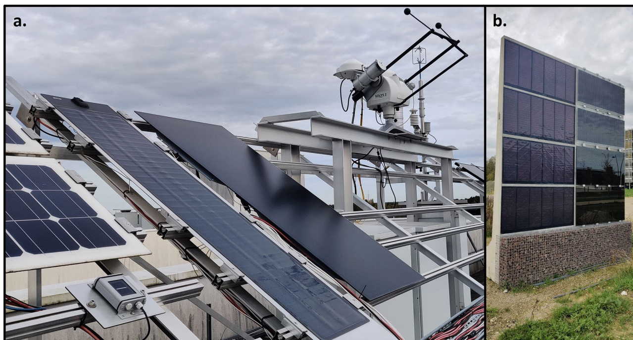
Fig. 2. Images of PV systems in Genk, Belgium used for validation of the model. (a) rack-mounted PV system containing a flexible CIGS module and a rigid CIGS module. This system is equipped with a weather station. (b) Concrete sound barrier with flexible CIGS modules.
