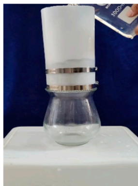
Figure 4. Illustration of the setup of the water permeability test.
