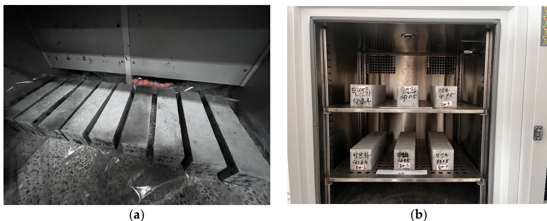
Figure 8. Carbonation specimens in carbonation chamber. (a) Carbonation specimen; (b) carbonation.
