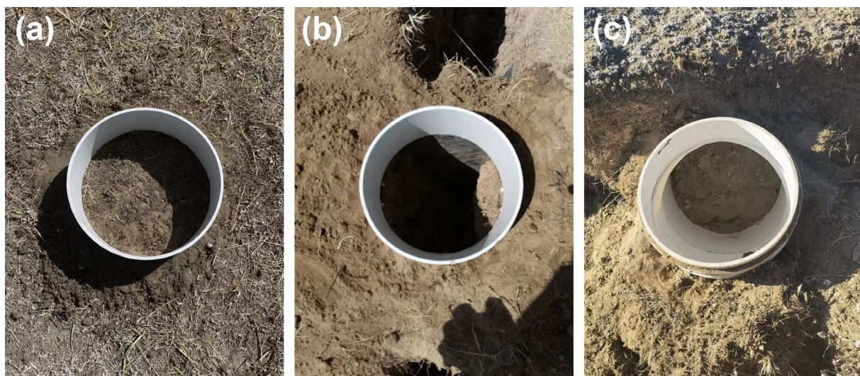
FIGURE 2 | Design of the carbon emission measurements from fissures created in the Maduo earthquake. (a) The control group (carbon emissions from a land surface without fissures). (b) The test group (carbon emissions from a fissure with a width of 20 cm and depth of 40 cm). (c) The test group (carbon emission from the fissure sidewall; the fixed base for measuring was a 90° elbow with an inner diameter of 20 cm).
