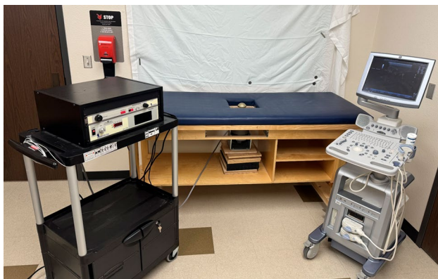
Fig. 1 The instrumentation required: shaker calibrator (left), shaker apparatus positioned under a modified measurement table (center), ultrasound device and transducer (right)
