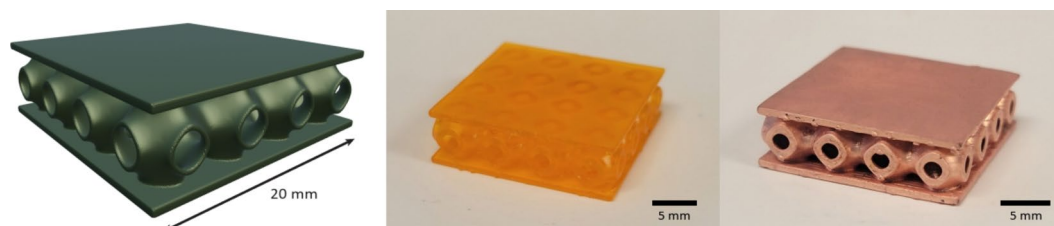
Fig. 8. TPMS lattice samples used for compression and conductivity tests. (a) CAD model lattice samples. Images of (b) as-printed and (c) Cu-plated samples.
