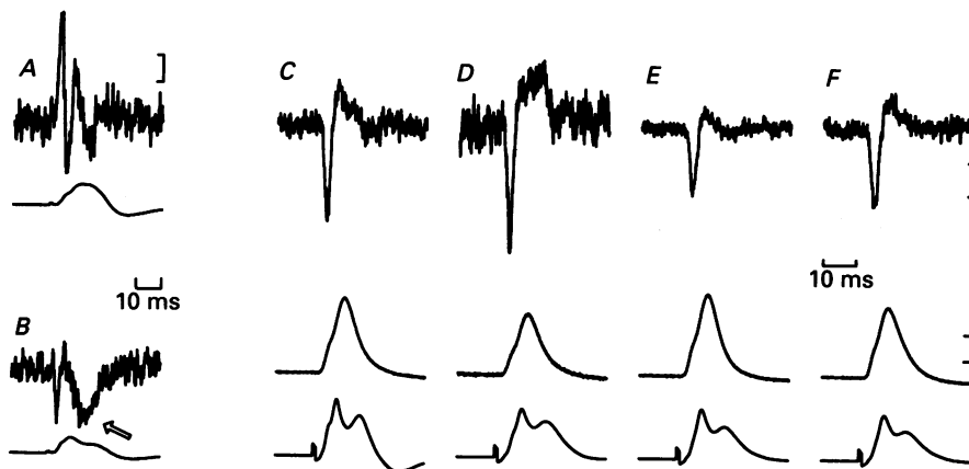
Fig. 13. Effects of stretch and change in wavelength on the optical rotation signal. A and B show an example in which stretching the nerve changed the polarity of the optical rotation signal. A , stretch 0%. B , stretch 7%. Upper traces, optical rotation signal. Calibration in A represents 5 \times 10^{-5} deg. A slow negative deflection in B (arrow) probably came from the birefringence change. Proximal stimulation. 550 nm. Resting retardation in the stretched state was 54 deg. 9 °C. C-F , effects of change in wavelength. C , 550 nm. D , 450 nm. E , 650 nm. F , 550 nm again. Top traces, optical rotation signals. Calibration in F , 5 \times 10^{-5} deg. Middle traces, birefringence signals. Calibration in F , 2 \times 10^{-4} of the background light intensity. Lower traces, externally recorded action potentials. Proximal stimulation. Resting retardation, 97 deg at 450 nm, 76 deg at 550 nm, and 63 deg at 650 nm. 11–12 °C.
