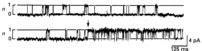
Fig. 4. Non-stationary gating of S-channel in an inside-out patch; n is the number of channels open. Top and bottom traces are continuous in time. Arrow in bottom trace marks transition of channel to high probability mode. Channel open probability was 0.35 before the switch, and 0.78 after it. Probabilities estimated from 12 s stretches of data. Membrane potential held at 0 mV. Current records filtered at 1 kHz.
