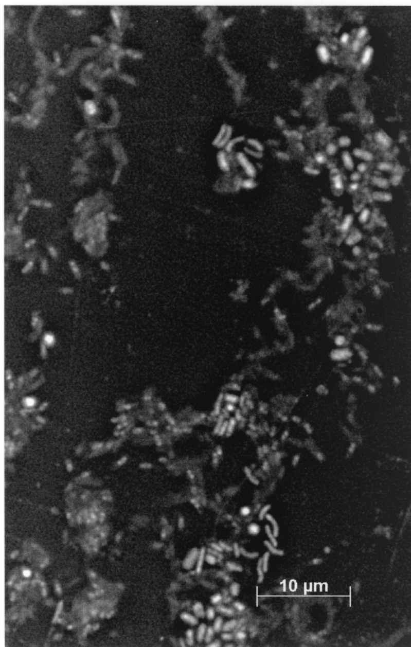
FIG. 3. Mixed-species heterotrophic biofilm grown on stainless steel in a potable-water biofilm reactor containing Pseudomonas aeruginosa , Klebsiella pneumoniae , and Flavobacterium spp. This image of a biofilm was obtained, after staining with 4',6'-diamidino-2-phenylindole, with a Zeiss Axioskop 2 epifluorescence microscope and the Zeiss deconvolution system.
