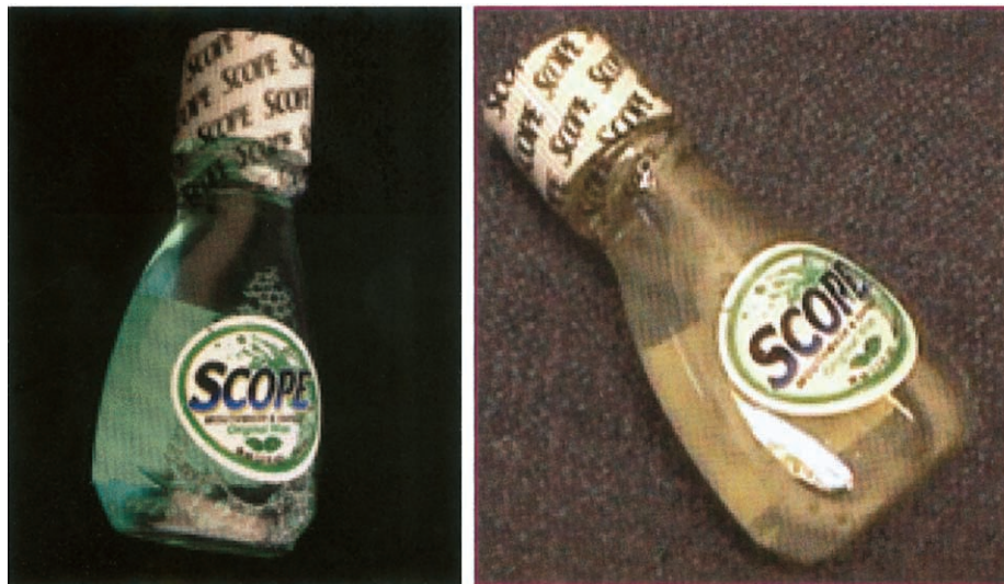
Figure 1 Color of Scope before (left) and after (right) sterilizing E-beam irradiation
