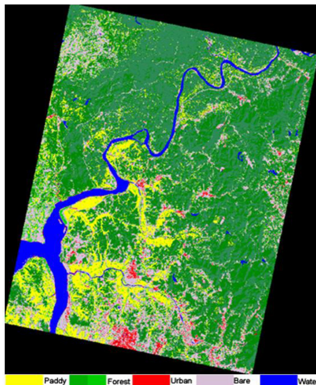
Figure 5 Land-use/land-cover classification of Paju District. Image was acquired on 10 September 2002. Rice paddy, forest, urban, bare land, and water are depicted by yellow, green, red, gray, and blue, respectively.
