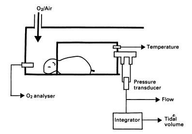
Fig. 1. Schematic drawing of equipment for ventilatory recordings. Ventilation was assessed from the flow passing in and out of the body plethysmograph via a pneumotachometer coupled to a pressure transducer. Inspired air could be switched to oxygen by means of a hood placed over the plethysmograph. Box temperature and inspired  $O_2$  levels were continuously monitored.
