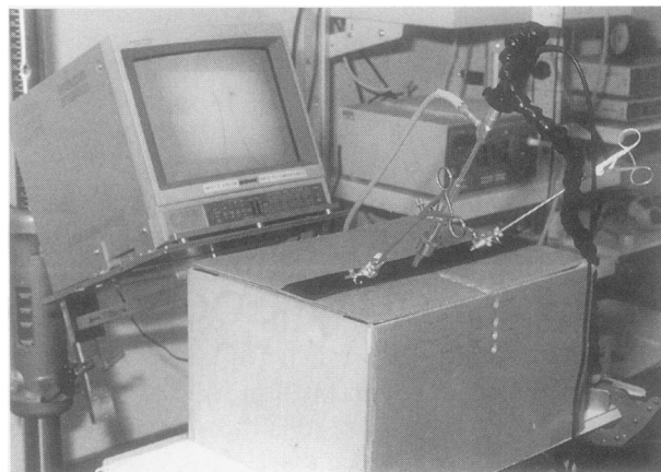
Figure 1. Experimental setup with the monitor in front of the surgeon at the manipulation workspace to allow gaze-down viewing by the operator.
