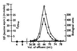
Fig. 3. Chromatography of 2300 'units' of bradykinin on a second column (0.9 cm.  $\times$  15 cm.) of Amberlite IRC-50. The effluent was collected in 0.9 ml. fractions.  $\triangle$ , Ninhydrin colour value;  $\bigcirc$ , light-absorption at 270 m $\mu$ .;  $\bigcirc$ , biological activity.
