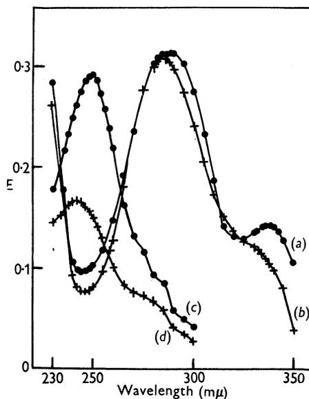
Fig. 6. Absorption spectra of aldehydes and acids. Each compound was dissolved in *m*/15 phosphate buffer, pH 6.98, to give a concentration of 0.02–0.03 *mm*. (a) 4-Hydroxy-3-methylbenzaldehyde; (b) 4-hydroxy-2-methylbenzaldehyde; (c) 4-hydroxy-3-methylbenzoic acid; (d) 4-hydroxy-2-methylbenzoic acid.
