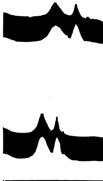
Fig. 2. Electrophoresis pattern of actin preparation from uterus muscle. Electrophoresis for 100 min. and 140 min. at 5.4 v/cm. Medium: 0.1 M-KCl–0.1 M-glycine, 67 mM-HCl, pH 2.35; concn. 6.6 mg./ml. Ascending boundary.
