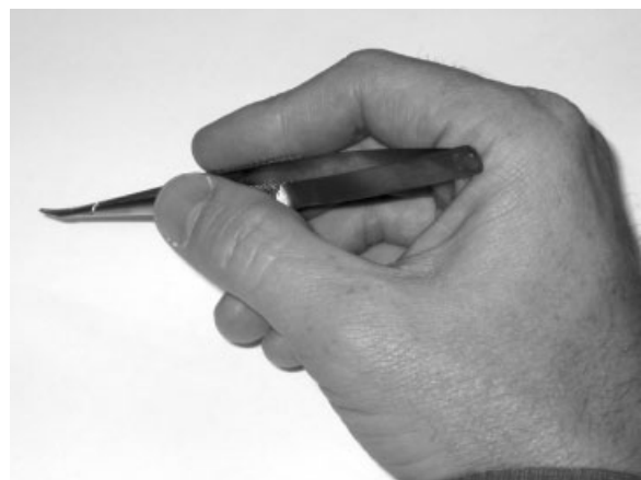
Figure 3 Basic position for holding the instrument. The thumb and index finger grasp the tool while the middle finger supports it from behind.
