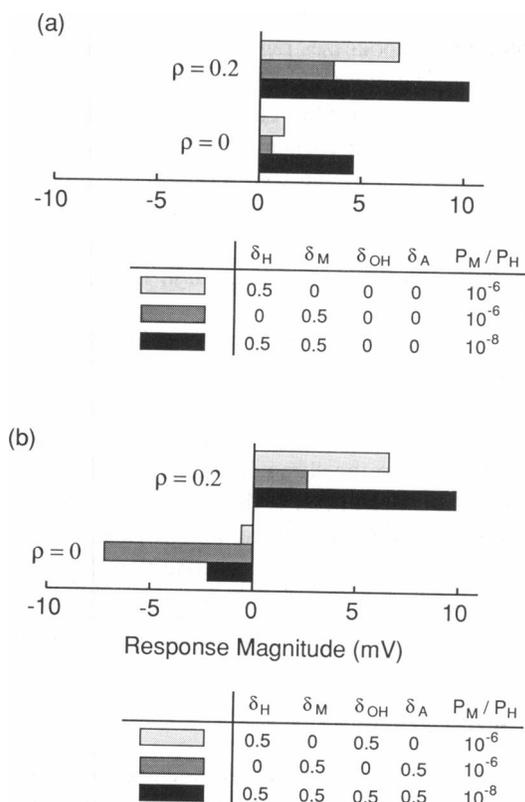
FIGURE 5 Response magnitude of the membrane potential as a function of the fraction  $\rho$  of the ionizable lipids in the membrane. Solutions are symmetric and contain 0.1 M of salt. pH is 7.  $\psi_p = 10$  mV,  $\theta_H = 0$ ,  $\theta_M = -0.5$ ,  $\theta_{OH} = 0$ , and  $\theta_A = -0.5$ .
