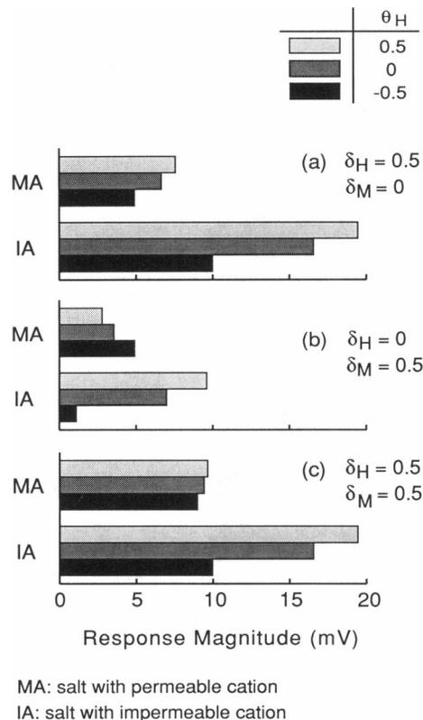
FIGURE 2 Calculated response of the membrane potential as a function of the relative changes  $\delta_H$  and  $\delta_M$  in the cation partition coefficients and the relative change  $\theta_H$  in the diffusion constant of the proton. Solutions are symmetric and contain 0.1 M of salt. pH is 7.  $\rho = 0.2$ ,  $\psi_p = 0$ ,  $\delta_{OH} = \delta_A = 0$ ,  $\theta_M = -0.5$ ,  $\theta_{OH} = \theta_A = 0$ , and  $P_M/P_H = 10^{-6}$ .
