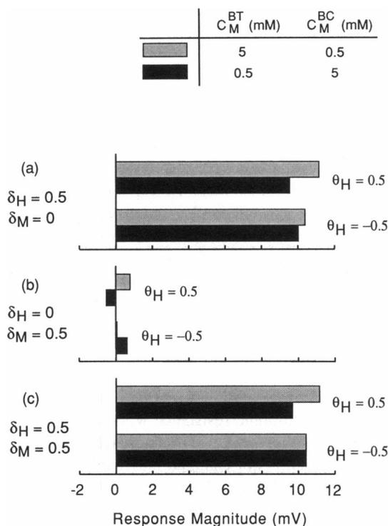
FIGURE 4 Comparison of the direction of polarization in the case where the salt concentration in *cis* side solution is higher than that in *trans* side solution, with the polarization direction in the case where the salt concentration in *trans* side is higher than that in *cis* side. pH is 7 in both *trans* and *cis* sides.  $\rho = 0.2$ ,  $P_M/P_H = 10^{-6}$ ,  $\psi_p = 0$ ,  $\delta_{OH} = \delta_A = 0$ ,  $\delta_M = -0.5$ , and  $\theta_{OH} = \theta_A = 0$ .
