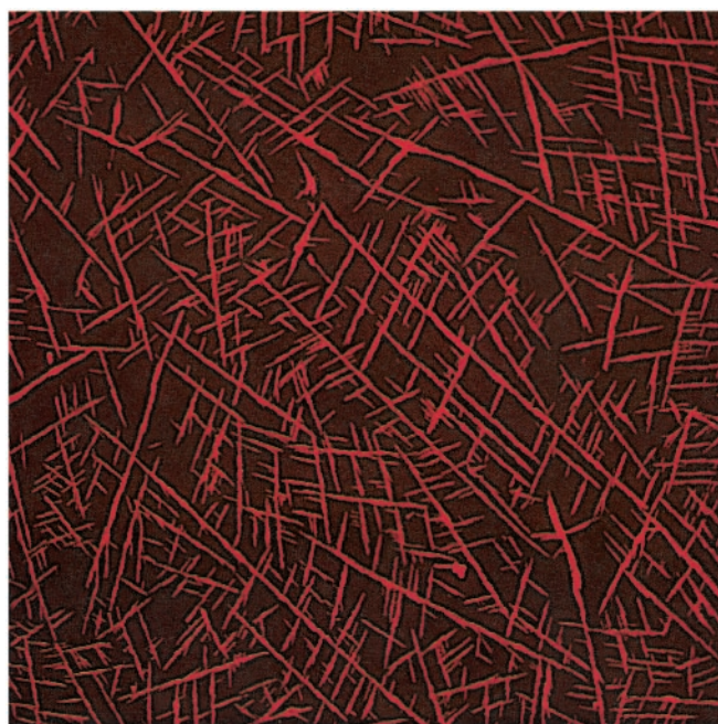
Fig. 2. Luminescence microscopy image of a microstructured thin film of the rhenium form of complex 1.
