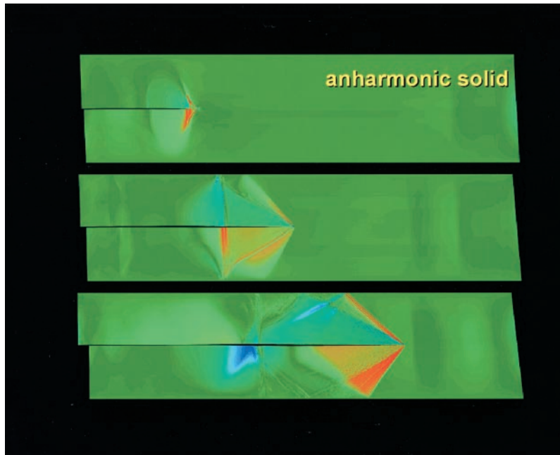
Fig. 4. Snapshot pictures of a crack traveling in the anharmonic slab, where the progression in time is from the top to the bottom. The boxed snapshot pictures represent a progression in time from the top to the bottom.
