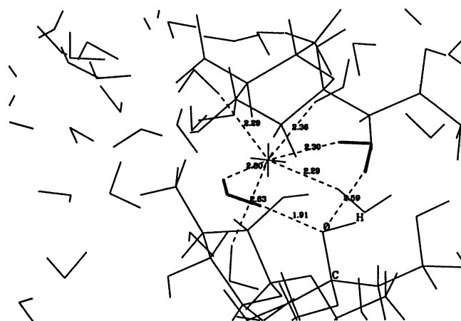
FIGURE 11 Snapshot of the solvent-shared complex at the entrance part of the pore. The hydrated anion is located in the vicinity of the OH-2 ligand. Two shared water molecules are represented by thick lines.
