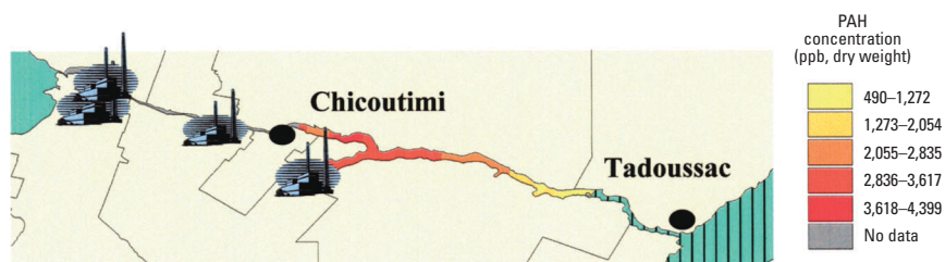
Figure 5. Saguenay River, Québec, Canada. Polycyclic aromatic hydrocarbon concentration in sediments (parts per billion, dry weight) (43). Chimney icon: aluminum smelters.
