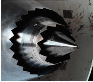
Just plane brilliant? Chevron nozzles (above) reduce the sound of exiting jet engine exhaust.
