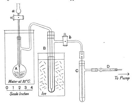
Vacuum Apparatus for the Distillation of Small Quantities of Ammonia.
