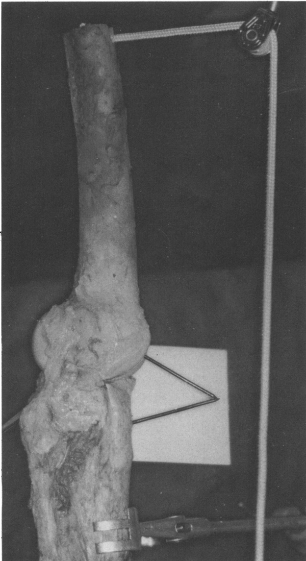
Fig. 2. Experimental arrangement: fixed tibia, nails inserted in femur and tibia (see Fig. 3), moment applied to the femur.
