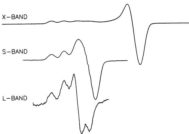
FIGURE 1 Multifrequency EPR spectra of the cupric site of azurin. Spectrometer conditions: X-band (9.13 GHz), 7.4 K; S-band (2.38 GHz), 120 K; L-band (1.14 GHz), 120 K; modulation amplitude, 5 G; modulation frequency, 100 kHz.
