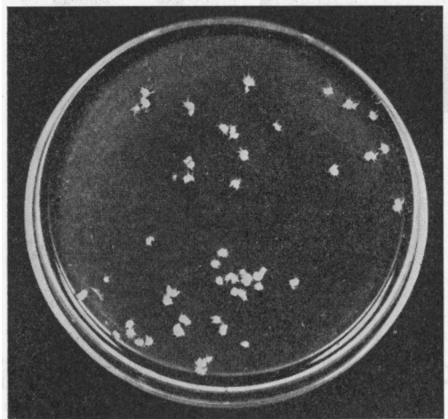
Fig. 7. Stellate gel bodies formed in swirled reaction mixture. Conditions standard except that mixture was agitated by swirling. Suspension was photographed in a Petri dish against a dark background at reaction time 4 hr. Note the fine radial arms. \times 0.8 .
