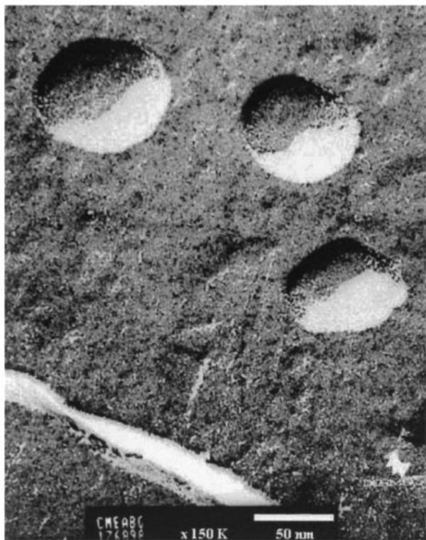
FIG. 1. Cryo-fracture transmission electron microscopy of cationic polysaccharide nanoparticles (PSP). Samples were frozen at -200^{\circ}\text{C} and cryo-fracture was performed at -150^{\circ}\text{C} on a Reicher-Jung Cryo-fract. Transmission electron microscopy was performed on a JEOL 1200 EX. Magnification, \times 150,000 .
