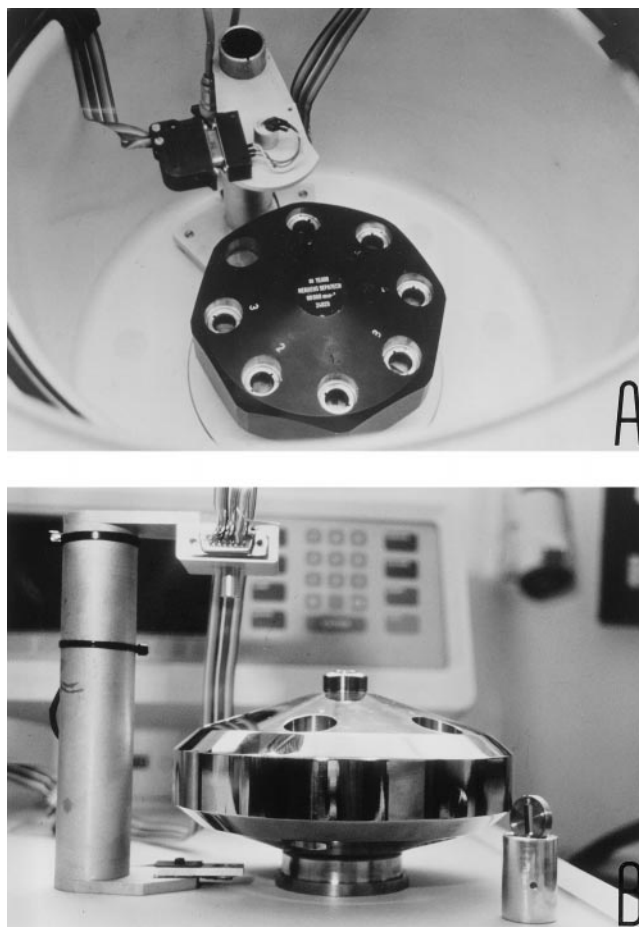
FIGURE 1 (A) Vacuum chamber of a preparative UC modified for use in PSD determinations. The eight-hole rotor shown here was custom-made by Heraeus. However, the An-50 Ti analytical rotor also could be used. The laser and detector optics are mounted to the vacuum chamber base using a mounting hole used to fasten the heat sink. The rotor can be lifted in and out of the chamber without disturbing the optics. (B) Laser-optical setup removed from the chamber. The rotor and a cell also are shown. The configuration is such that in operation the laser diode light source is above the rotor and the photo diode detector is below the rotor. The elliptical laser beam is collimated. A 2 mm \times 0.2 mm slit on the bottom window of the cell defines the source beam used for turbidity analysis. As there is very little distance between the slit and the detector, little diffraction broadening of the beam can occur. This arrangement results in a very narrow acceptance angle by the detector, thus ensuring that light scattered at low angles ( 10^\circ ) will be excluded from detection. Thus, effects of stray light are minimized.
