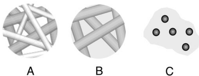
FIGURE 5 Idealized structures of composite gels. (a) A matrix of randomly oriented agarose and dextran fibers with water-filled interstices. (b) A homogeneous dextran gel with agarose fibers acting as barriers. (c) A homogeneous agarose gel with dextran spheres acting as barriers.
