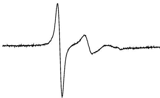
FIGURE 3 CW Q-band spectrum of 100- \mu M arrestin K267C-MTSL. The 100-G spectrum was signal averaged four times at a power of 0.2 mW with a 120-s scan time, 0.1-s time constant, and 1.25-G modulation.
